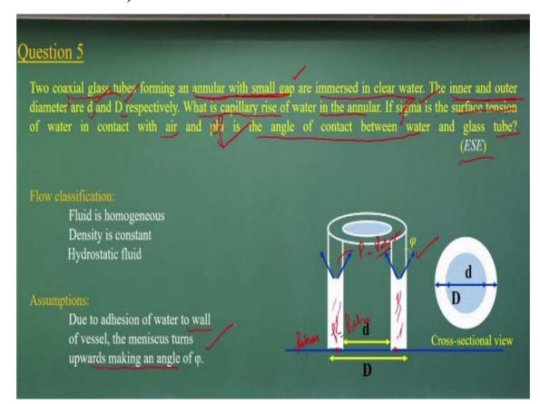
Now let us go to the question number 5 which talking about the capillarity and the surface tensions. So this is what the Engineering Service exam paper where the two coaxial glass tubes forming a annular with a small gap okay. There will be annular but the gaps are small immersed in a clear waters. The inner and the outer diameters are small d and the capital D respectively.
