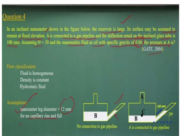
Now let us come it to a manometer problems. So there is a inclined manometer shown in the figure below. Reservoir is large. That is the, its surface maybe assumed to be remain as a fixed elevations. A is connected to a gas pipeline. The deflection is noted on the inclined gas tube. This is what the inclined gas tube is 100 millimeters the theta the angle of inclined manometers theta equal to 30 degrees and manometric fluid as oil with a specific gravity of 0.86.
