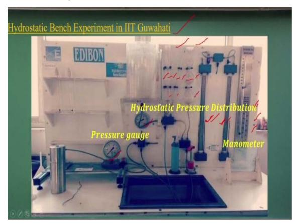
Now let us look at the hydrostatic bench experiment setup, which is there in IIT Guwahati. So this type of experimental setups which is called this hydrostatic bench experiment setup, you can see the pressure gauge, you can see the pressure gauge. You can see this mercury manometers. So these are mercury manometers are there. These are U-tube manometers are there.
