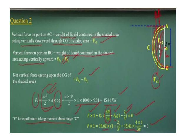
Similar way if I need to compute the how much vertical force is acting on this. So we can find out if this is my free surface. This is the area, the shaded part will give a vertical force component of  $F_{v1}$ . But  $F_{v2}$  will be the, all the shaded part will be the  $F_{v2}$  part. The subtracting this part that what will be the net force what will be act vertically upward directions.
