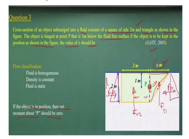
Now let us come to the another questions number 3, the cross sections of object submerged into a fluid consists of a square side of 2 meters and the triangle as shown in the figure. Object is hinged at the point P is 1 meter below the fluid free surface if object is to be kept in this position as shown in the figure, the value of x should be what is the x value so that this will be at a same position, the equilibrium positions.
